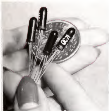
Single transistors of the 1950's – based on germanium.
